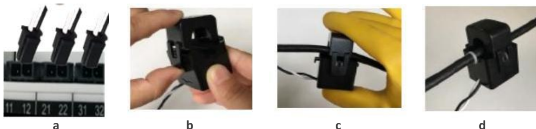
Figure 2-15 5A/2mA, 50A/40mA, 100A/40mA, 200A/40mA or 400A/40mA SCCT Installation
